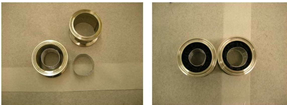
Fig. 2-4 Empty cylinders (on left) and cylinders with “rings” of activated carbon along side walls.
