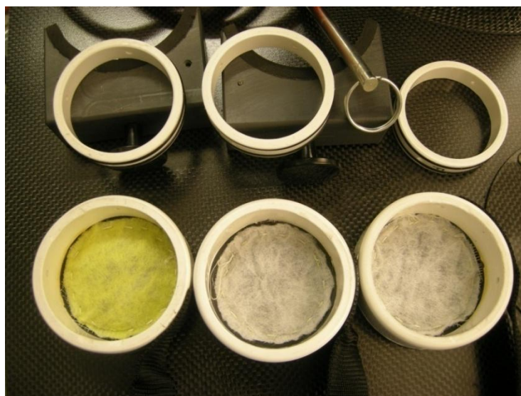
Fig. 2-23 Installation of filters for particle removal performance test.
